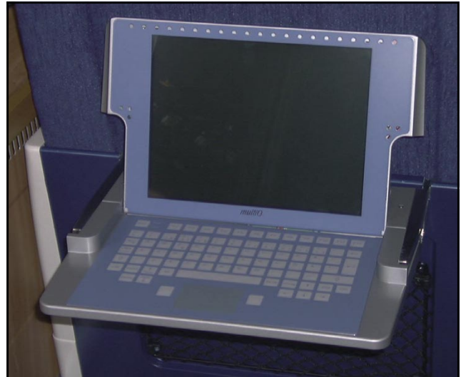
A Custom InduKey® Short Travel Keyboard, build into a Swedish High Speed Trains
