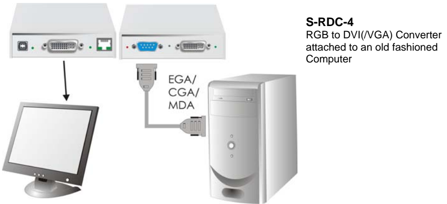
Figure 20 RGB to DVI(/VGA) Converter with optional EGA/CGA support, attached to an old fashioned Computer
